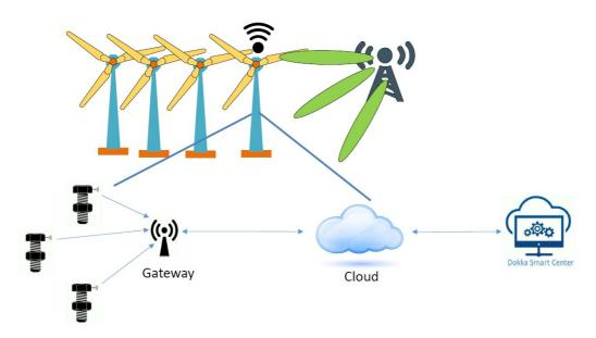
SMART BOLTS DEVELOPED BY DOKKA FASTENERS WITH COLLABORATORS AT NTNU GJØVIK CAN ENABLE SAFER WIND TURBINES AND REDUCED MAINTENANCE COSTS(REI
