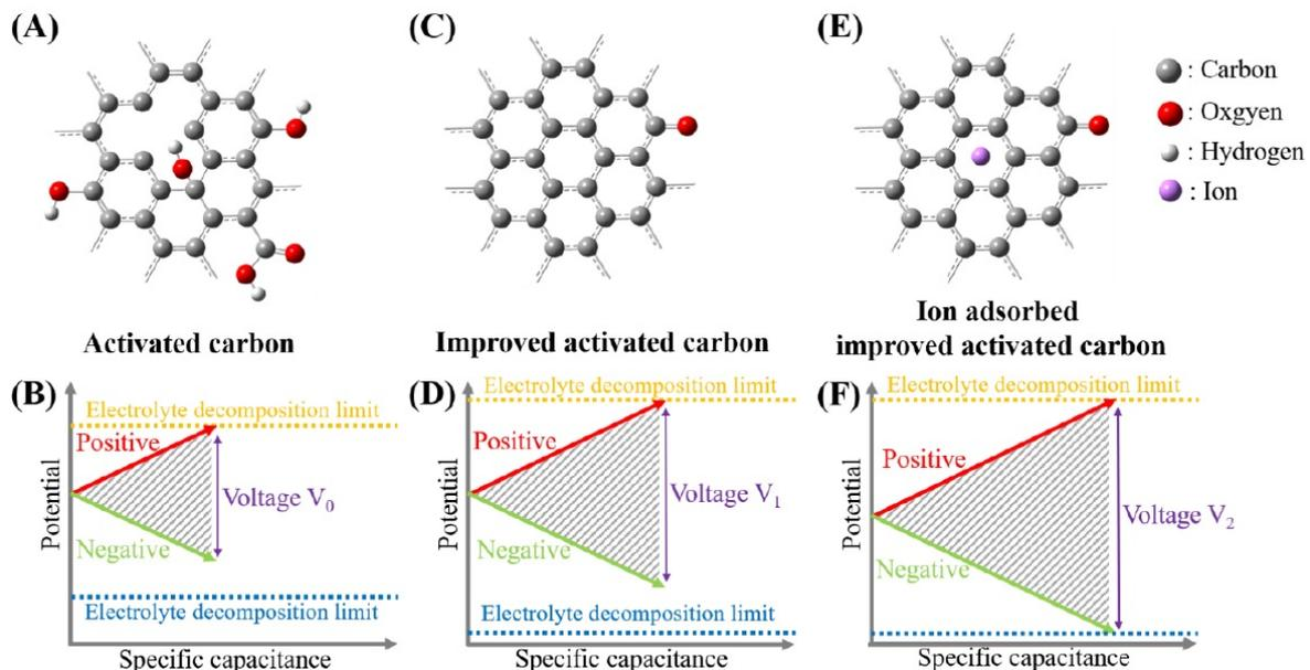
**Figure 1.** Approaches to widen supercapacitor operating voltage window by activated carbon modification
